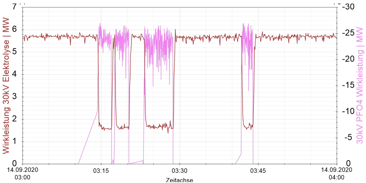
Figure 9: graph of measured power of LAF No.4 and the AC power of the electrolyser
