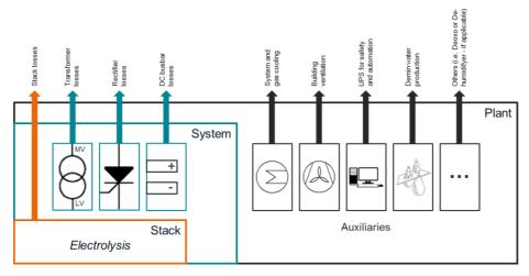
Figure 1: Electrolysis stack-, system- and plant levels
